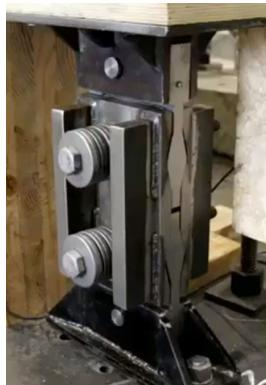
As shown, the RSFJ hold-downs were installed in the notches at the bottom corners of the CLT wall. The RSFJ configuration was composed of two centre slotted plates and two cap plates.
