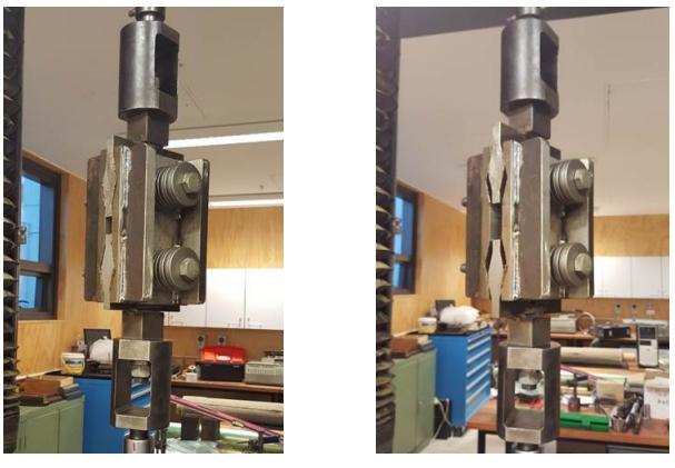
The displacement schedule with an average loading rate of 0.5 mm/s was applied to the specimen with different prestressing forces and different deflections. The schedule which is based on the previous experiments carried out on the similar slip friction connections includes four reverse cycles at 20%, 40%, 67% and 100% of the maximum targeted displacement. A sample hysteresis response of the joint is shown below demonstrating the damping and self-centring capacity of RSFJ.
