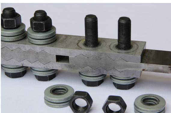
The lateral resistance of this new joint is higher than conventional flat plates friction joints for a similar clamping force provided by high strength bolts.
