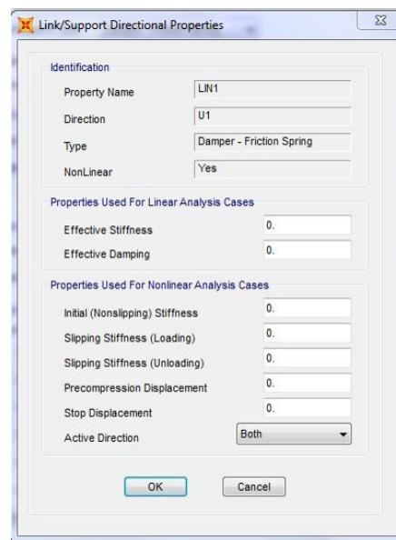
In SAP2000 the RSFJ load displacement behaviour can be easily modelled by choosing the Damper-Friction spring type link element.
